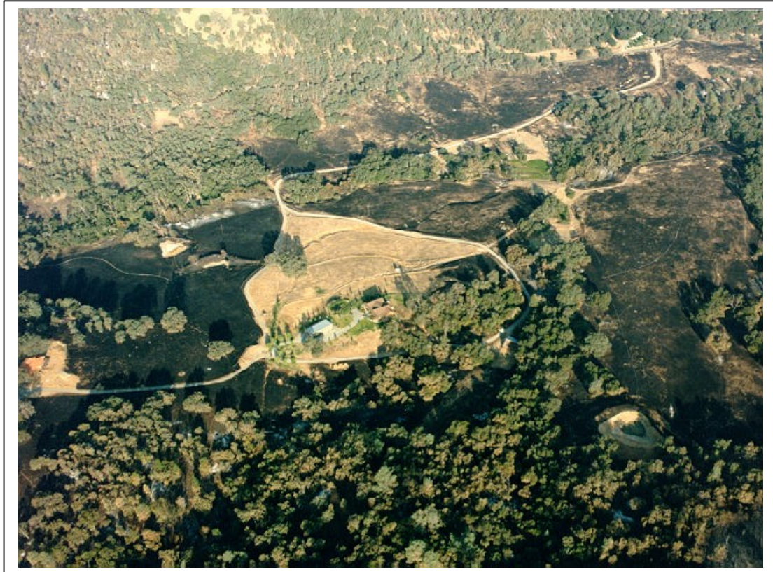
Photograph 10.1. House Showing Defensible Space
